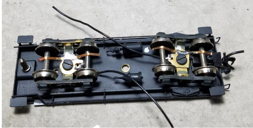
Photo 3: The phosphor bronze wiper and wire have been soldered to each piece of brass and the trucks have been reinstalled. Be sure to keep the insulated wheels on the proper side or a dead short will have been created!
